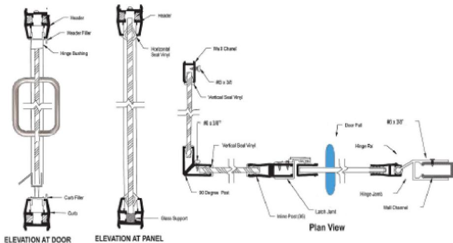
17. Stand inside shower and hold the straight edge on outside of wall channel, in-line post and 90-degree corner post above door. Holding them in line, pull door closed and align to latch jamb by moving the 90-degree corner post (17) in and out at top of the 90-degree panel
